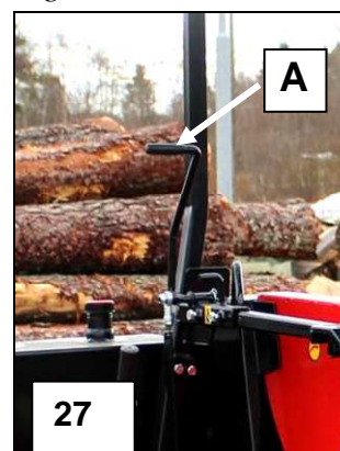
Fig. 27. Tightening and slackening of the V-belts
