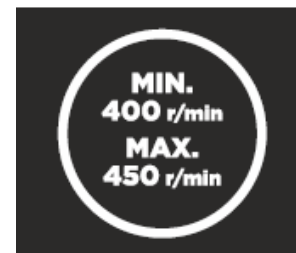
Revolutions range for PTO-shaft
