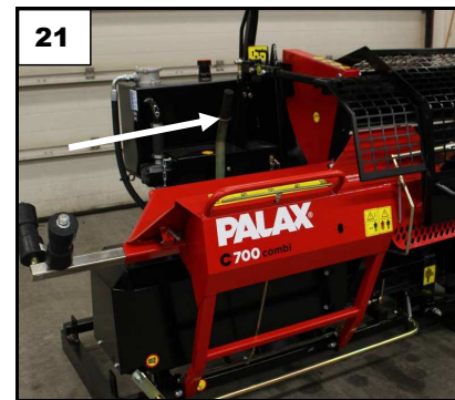
Fig. 21. Manual starter for the splitting operation
