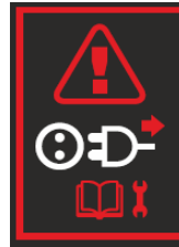
Disconnect the machine from the electric supply before taking to any service measures
