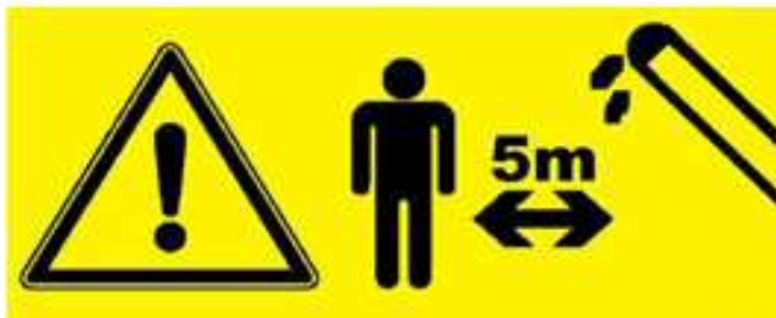
Safe distance from the conveyor 5 m
