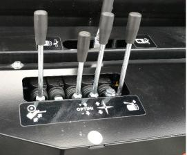
Control of the log table as it appears in varying control panels. The controls are marked on the log deck with illustrative symbols.
