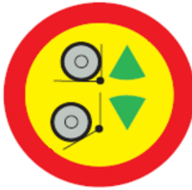
Manual operation of the dropping plate
