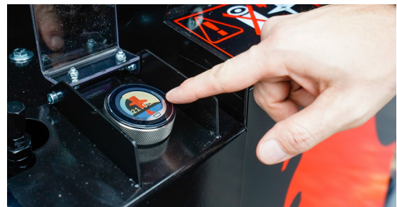
With X-Aim's intelligence, the user also gets real-time data on work productivity: the touch encoder distinguishes processed cubes, hours of operation, number of cycles and saw squares.
