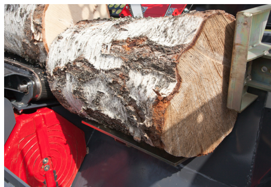
The dropping plate guides the wood straight into the splitting chute.
