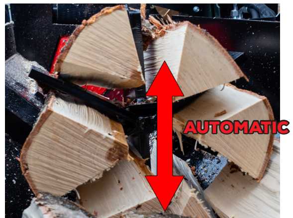
X-Aim automatically adjusts the splitting wedge to the optimum height in the middle of the log.
