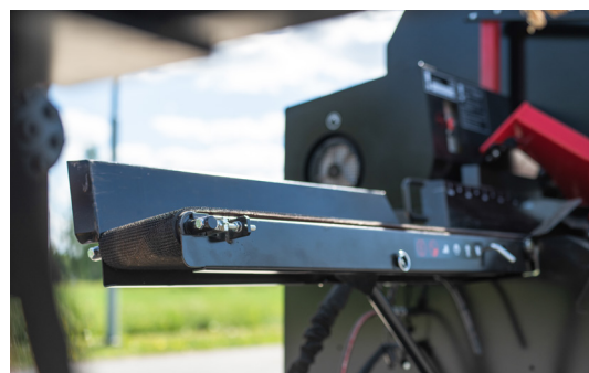
A solid backboard of the in-feed conveyor eases log feeding.
