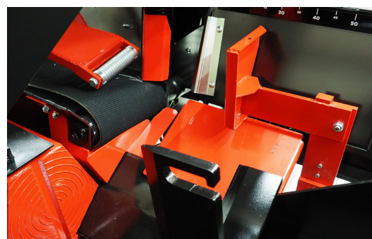
The dropping plate guides the wood straight into the splitting chute.
