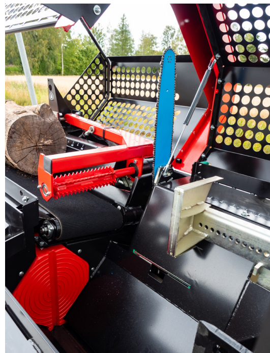
The log clamp with a hydraulic drive roller ensures efficient log feeding.
