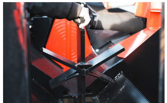
Changing the splitting wedge is quick and easy.
