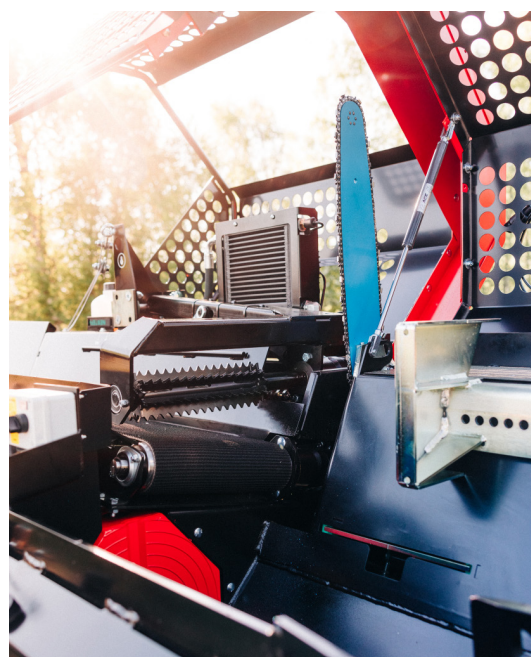
The log clamp with a hydraulic drive roller ensures efficient log feeding.
