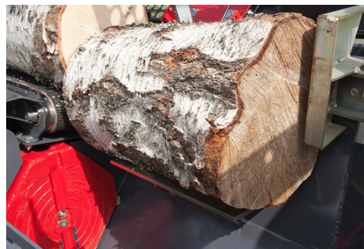
The dropping plate guides the wood straight into the splitting chute.
