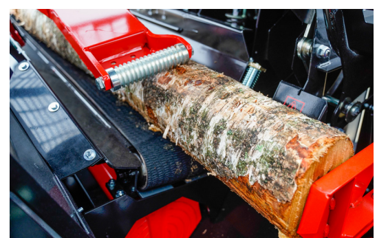
The hydraulic log clamp works automatically and improves log control.
